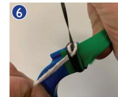
Pull the loop material back underneath the final two wraps. If you have a long piece of wrap material over-hanging you can always trim it back with a sharp pair of scissors.
