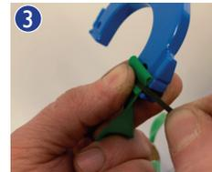
Fold the excess band material back over your wraps & wrap another two times. Always keeping the wrap material tight.
