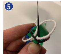
Carefully holding the tensioned wraps in place, feed the end of the wrap material through the loop.
